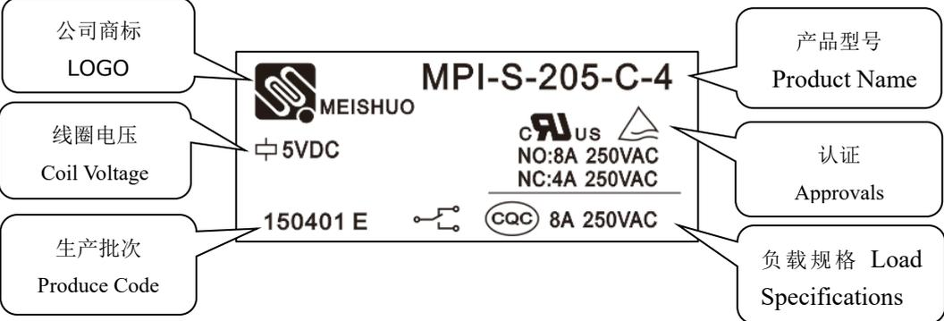
The diagram shows a relay label with the following markings and their corresponding callouts:
