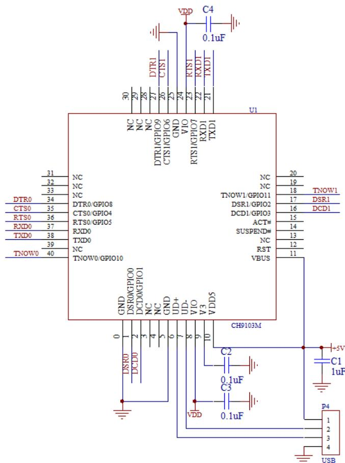
The figure above is the USB to TTL converter realized by CH9103. Only RXD, TXD and public ground are necessary connection, while the others are optional.
