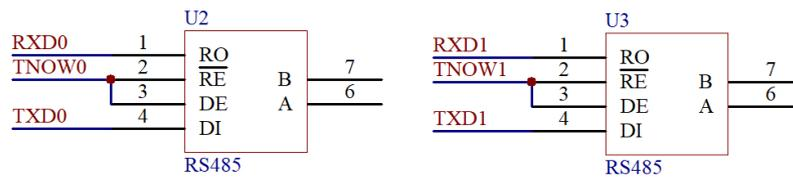
In the figure, TNOW is the switch pin, the TNOW pin can be used to control DE (active high and transmit enabled) and RE# (active low and receive enabled) pin of RS485 transceiver. RS485 transceiver should use the same power supply as VIO.
