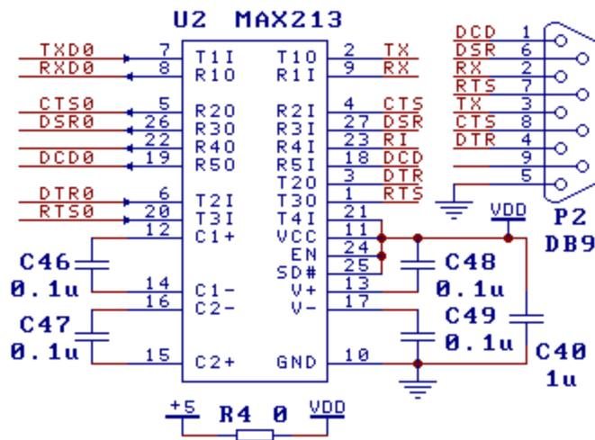
CH9103 provides common UART signals and MODEM signals, converts one of TTL to RS232 through level conversion chip U2, the other one is similar with this. Port P2 is DB9 connector, the pins and their functions are the same as common PC DB9 connector, the chips similar with U2 have MAX213/ADM213/SP213/MAX211 etc. U2 in the image is uniformly powered by the USB bus through R4.
